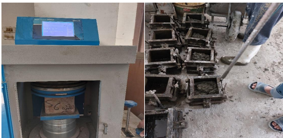
Figure 4. Molding and testing of standard compressive strength cubes
